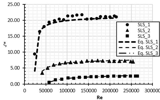
Figure 5. Measured and predicted frictional coefficient of slotted sieves versus Reynolds number
