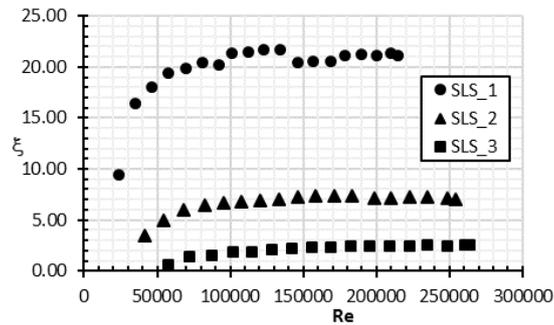
Figure 4. Frictional coefficients measured on slotted sieves versus Reynolds number
