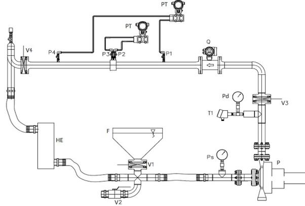
Figure 3. Experimental test rig. HE – heat exchanger; P – centrifugal pump; Ps, Pd – suction and discharge pressure; PT – pressure transducer; p1, p2, p3, p4 – pressure taps; Q – magnetic flow meter; T1 – thermocouple; V1, V2, V3, V4 –feeder, drain, discharge and check valves
