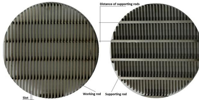
Figure 1. Slotted sieve used in experiments; to the left - front side; to the right - backside
